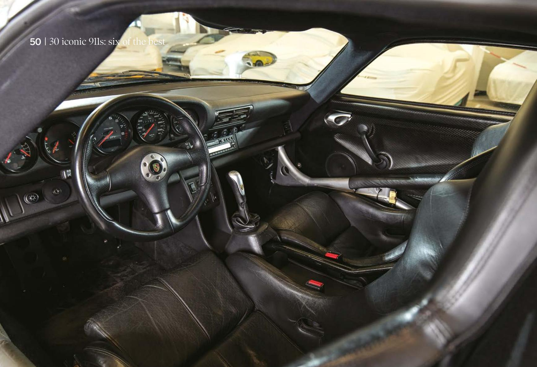
**Above** Inside the GT1, the steering wheel, dashboard, five dials, gearlever and even the seats are all reminiscent of a 993 RS specification. Note the 996-generation door handles, however
