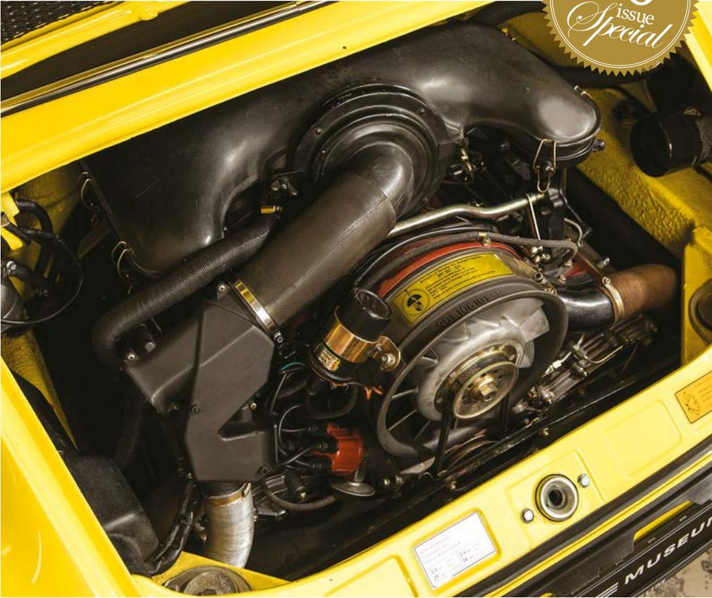
**Left** The 2,687cc engine produced 213hp and 255Nm of power and torque respectively, achieving a top speed of 152mph and a 0-62mph time of 5.8 seconds – sprightly for 1973
